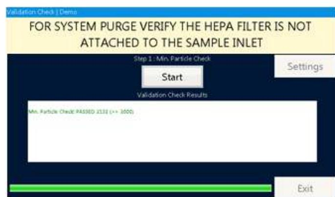
Remove the HEPA filter or the mask if attached, and tap the [Start] button to check that the particle concentration in the ambient air is sufficiently high enough to calculate the mask fit factor. Depending on the ambient particle concentration (i.e., outside of the mask), the environment may be inappropriate to perform a mask fit test. This process also confirms that the device is operating properly. When this measurement is complete, proceed to the Zero Check
